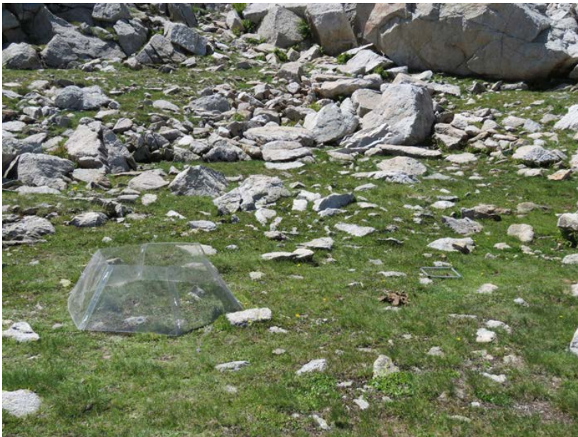
Figure 1. An Open Top Chamber installed in the Ratera snowfield.
